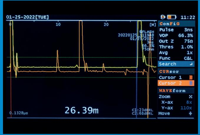
District heating application, finding where leaks have affected the insulation and therefore the VOP
