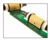
Precision by design A unique arrangement of five custom manufactured, precision ground antennas deliver locate accuracy and repeatability
